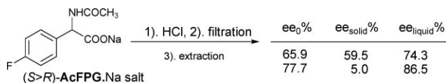
Fig. 18 Enrichment by partial precipitation of racemate forming AcFPG starting from the sodium salt of its enantioimpure mixtures.
